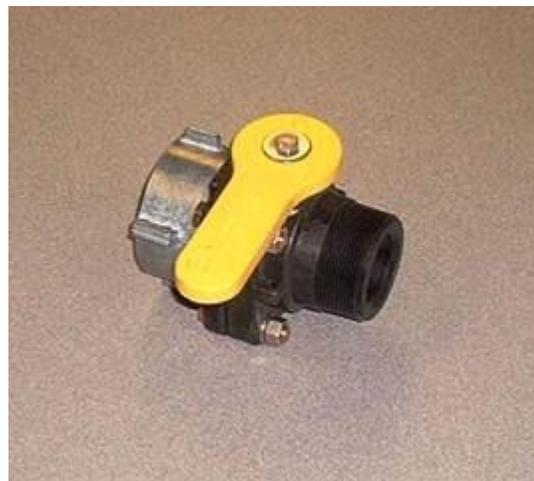
These next two pictures (above) identify the “OLD STYLE” Schuetz bottle. The valve has an independent metal collar which can spin to loosen or tighten the valve to the bottle.
