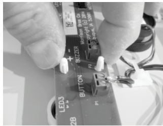
Figure 15 - Press the center of the Indicator Board completely down onto its supports
