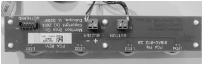
Figure 11 - Place the Indicator Board back in place on its supports
