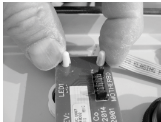
Figure 16 - Press the first end of the Indicator Board completely down on to its supports
