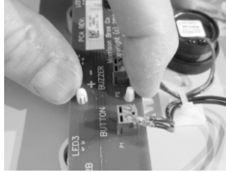
Figure 13 - Press the center of the Indicator Board partially down on its supports
