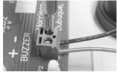
Figure 4 - Disconnecting the Buzzer from the Indicator Board
