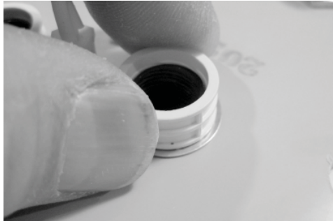
Figure 26 - Removing the Lens Nut from an existing Indicator
