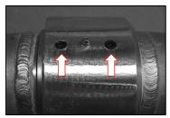
STEP 6: Reinstall the ball retainer screw until tight. If this prevents smooth rotation, back off 1/8 turn. A thread locking sealant is recommended to prevent screws from backing off. After pressure testing, the unit is ready for installation.
