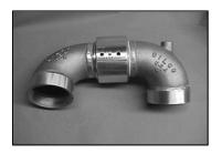
STEP 4: Insert the sleeve into the body while slowly rotating it into position. Take caution while applying force to pass the radial ball bearing grooves and seat the main pressure seal properly. If the sleeve becomes hung up, remove and re-insert, careful to maintain even pressure and plumb alignment.
