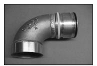
STEP 2: Install the new "O" ring on the sleeve (this is the product/pressure seal to be place up front – the initial contact of the body and sleeve). Then install the dust seal at the rear of the sleeve. For 80 Series, dust seal is felt material. For 880 Series, dust seal is rubber material.
