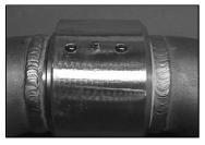
STEP 5: When the sleeve is fully inserted, feed the ball bearings into the raceways. Insert a flathead screwdriver (or bearing tool) and rotate the joint to make space for the balls (be careful not to damage the threads or scratch the raceway surface). Then reverse rotation to insert remaining balls.
