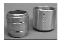
STEP 1: Remove the ball retainer screws. Add a sufficient amount of solvent into each raceway to flush out the lubricant. Rotate the sleeve, catching the balls as they fall out. When all the balls have been removed, the body and sleeve may be separated. Discard old seals. Thoroughly clean both body and sleeve.
