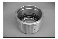
STEP 3: Lubricate packing seal area of body and then insert spring adapter and three v-ring seals.
