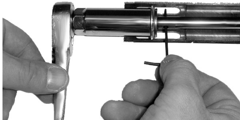
Fig. 1: Removing Grease Intake Assembly
