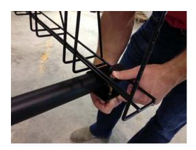
3. Place drip tray insert pans w/screen into the drip tray holder spaces.
