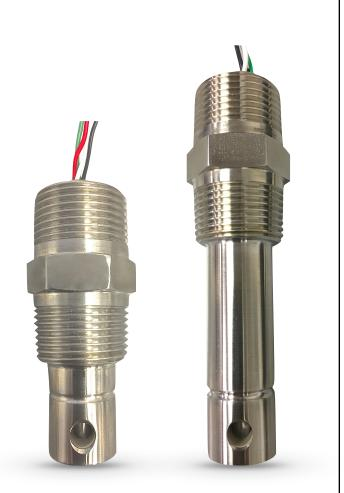
The ACS41 sensor was designed for high pressure, high-temperature conductivity measurements and is an excellent choice for boiler control and cooling tower applications. Blowdown control, condensate monitoring, leak detection on heat exchangers, and steam purity measurements are just a few of the many applications. The rugged one-piece body design provides a dependable sensor free from weld defects, including pinhole leaks.
