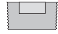
Fig. 2140 Bushings Flush Size Range: ¼" x ⅛" – 2" x ¼" (All sizes are POA)
