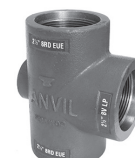
Pumping Tee Size Range: 2" 8RD EUE x 2" 8RD EUE x 2" 11 1/2" V REG - 3" 8RD EUE x 3" 8RD EUE x 3" 8V LP
