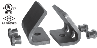
Fig. AF086 (Afcon Fig. 086) Adjustable Structural Attachment Size Range: Flange Thickness up to ½" thick (UL), up to ¾" thick (FM)
