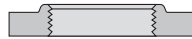
Fig. 1011 Cast Iron Companion Flange Size Range: Fig. 1011 ¾" x 3⅞" thru 12" x 19" NPS
