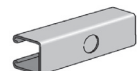
AS 300KO Channel with Knock Outs Size: 1 7/8" x 1 1/8" x 12 GA. 7/8" Knock Outs on 6" Centers.
