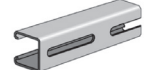
AS 210S Channel with Long Slots Size: 1 7/8" x 1 7/8" x 14 GA. 1 3/32" x 3" Slots on 4" Centers.
