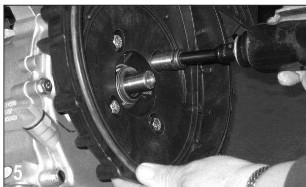
Remove the four bracket screws (12715A), rear bracket washers (12901), and screw head O-rings (12717) from the rear bracket using a 1/2" socket. With the four bracket screws removed, the rear bracket can now be removed from the drive unit.
