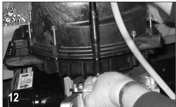
Install the pump body (12712/13712) as shown below with the outlet flange facing up. Install the 10 body screws (12720), 10 lock washers (V07018), and 10 nuts (V07019) to secure the pump body to the rear bracket. Tighten the bolts securely to 75-100 in lbs all the way around.
