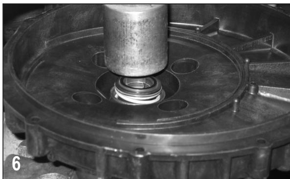
Remove carbon seal half from rear bracket with a round object. Tap gently with a hammer. Take care not to crack seal if reusing. Once disassembled; clean all reusable parts thoroughly, removing any traces of old gasket material and trapped / dried liquids from pump.
