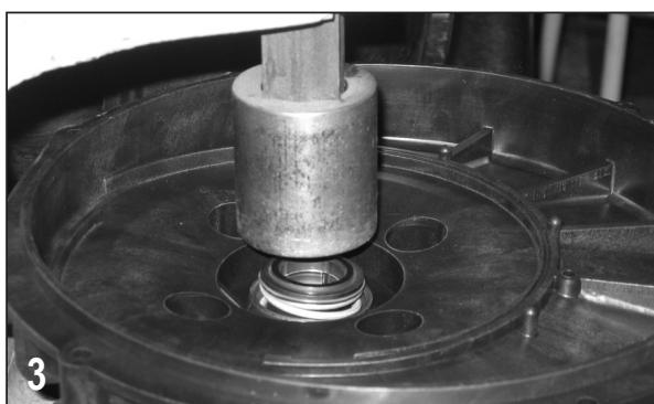
To install the carbon seal (12713) half into the rear bracket use a tool such as a 2" hose barb or arbor press to give even pressure on the metal flange of the seal housing during installation.
