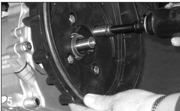
Install the rear bracket onto the drive unit using the bracket screw assemblies from the previous step. The handle of the rear bracket should be to the top of the drive unit. Tighten the screws securely to 125-150 in lbs.
