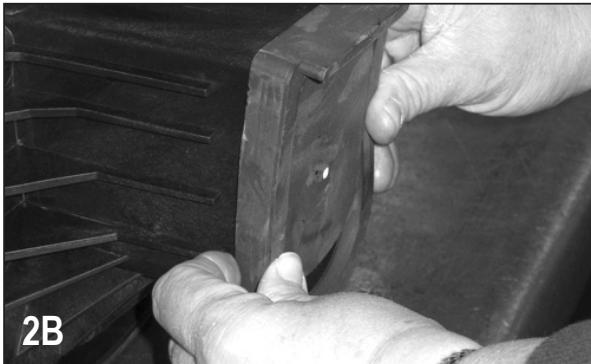
Remove the check valve (12705) from the volute (13702). Remove the one upper volute screw (12900) and the two smaller volute screws (12725) from the volute. Remove the volute from the remaining pump assembly.
