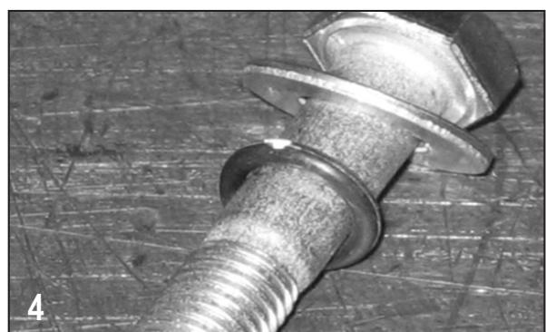
Clean the threads of the bracket screws (12715A) thoroughly. Once clean, install the four flat washers (12901) and four screw head O-rings (12717) onto each of the bracket screws.
