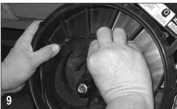
Install the O-ring segment (12754) onto the rear bracket as shown.
