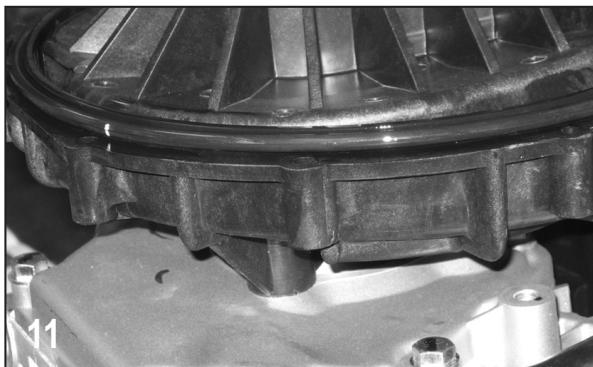
Place the pump body O-ring (12719A) around the outside flange of the rear bracket. The O-ring may be sparingly lubricated with silicone to ease installation of the pump body in the next step.
