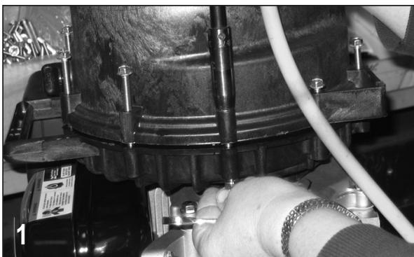
Remove the 10 body screws (12720), lock washers (V07018) and nuts (V07019) from the pump assembly. Remove the body from the pump assembly.
