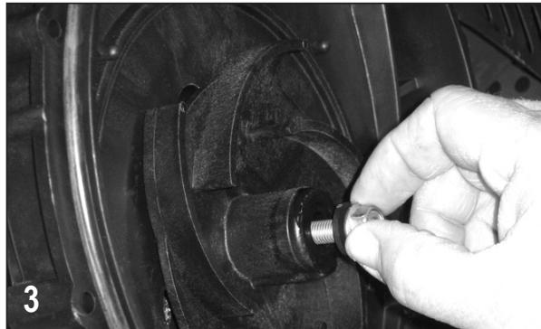
Remove the impeller bolt (12765A) from the impeller (12771A/12772). Remove the impeller bolt gasket (12774VA) from the impeller.
