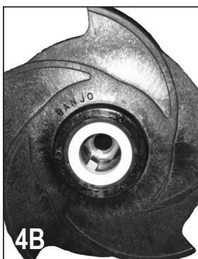
**4A:** Screw the supplied 7/16-14 hex head cap screw into the impeller snout. As the bolt is tightened the impeller will be pried off of the shaft of the drive unit. Remove the 7/16-14 screw once the impeller has been removed from the drive unit. **4B:** If the pump impeller is going to be reused the ceramic seal half (12713) should be removed from the impeller at this time. The impeller key (12902A) located behind the ceramic seal half should be replaced at this time also.
