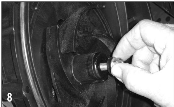
Secure the impeller to the drive unit shaft with the impeller bolt gasket (12774VA) and impeller bolt (12765A). Tighten the impeller bolt until snug (31-55 in lbs).
