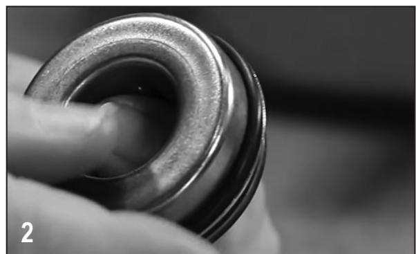
Place the seal O-ring (12710) behind the lip of the carbon seal half.
