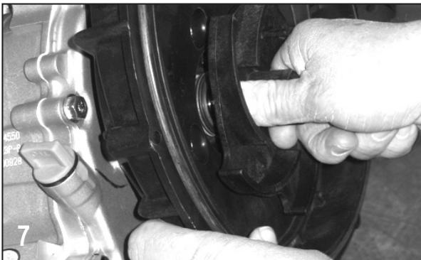
Place the impeller key (12902A) in the slot located inside the impeller snout. The impeller (12771A/12772/13772) is now ready to be slid onto the drive unit shaft. Be sure to align key with the keyway of the drive unit shaft.
