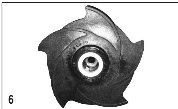
Verify impeller hex nut (12775A) is located at the bottom of impeller snout (should be installed). A very light press fit may be required to install nut into cavity. Install the ceramic seal half into hub of impeller by using an arbor press or similar tool. Outside diameter of rubber boot may be sparingly coated with silicone to ease installation.
