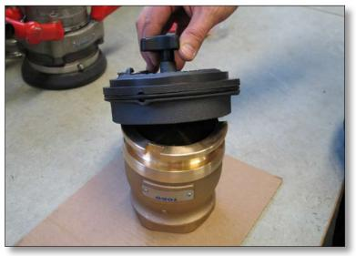
I) <u>Do not</u> use anything other than the handles provided to operate the couplings. The handles are specifically designed to provide sufficient assistance in operation.
