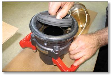
**k)** Ensure the tank unit cap (if fitted) is replaced and secure.
