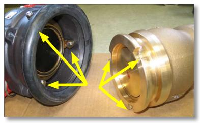
To allow the coupler to locate to the adaptor, and still supporting the hose assembly, rotate the coupler whilst gently pushing towards the adaptor. You will feel the coupler move forward about 1" (25mm).
