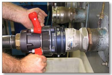
**h)** Still supporting the hose assembly, pull the coupler away from the adaptor. You may feel a small resistance due to seal vacuum.
