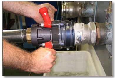
**d)** Still supporting the hose assembly, rotate the coupler clockwise about 100 degrees. At the start of rotation you will feel some resistance. The level of resistance is dependent upon the static line and tank pressure.
