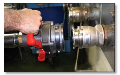
The handles have no operating purpose other than providing handling assistance, thus do not use tools, pipes etc. to assist connection.
