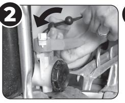
**Step 2** Press IBC Valve Cord Lock button in and slide down behind the IBC Valve leaving a 1" to 2" gap.
