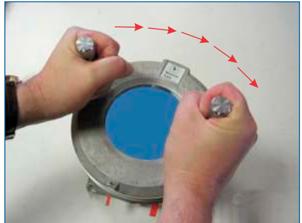
Lid fitting: With lid keys securely located in holes, rotate lid clockwise to tighten the lid onto the enclosure
