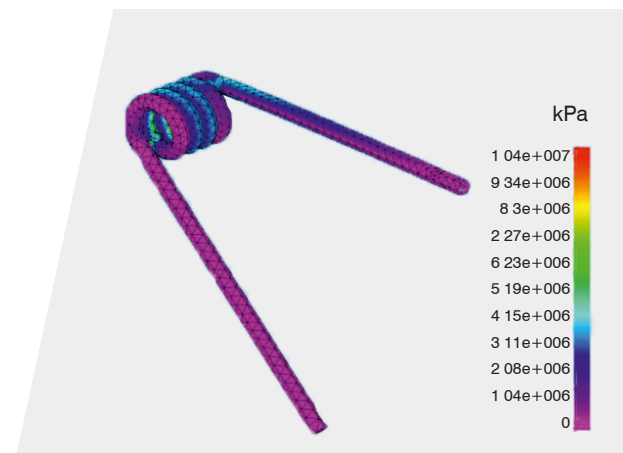
Newson Gale springs are designed and analysed with the aid of Finite Element Analysis technologies.
