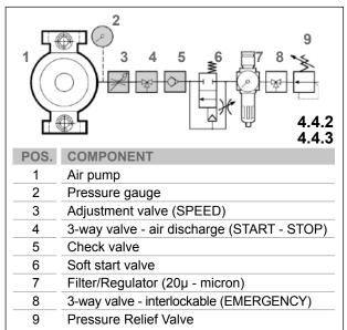
4.4.2 Tighten a compressed air flow control valve, a 3-way valve (START - STOP with air discharge) and a check valve on the pneumatic circuit connection of the pump, as per the diagram in the figure. Install a pressure gauge on the compressed air connection of the pump itself and check the value with the pump running to check the real pressure of the supply air.
