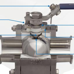
Belleville washer and 3-piece packing design adjusts for wear and temperature fluctuations
