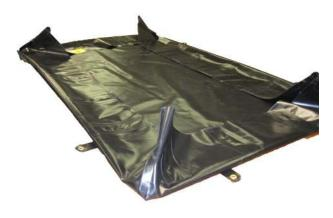
3. Slide L-brackets into the Berm pockets to support the sidewalls. Do this for all but the one wall that will be used to load the spill pallet and IBC. (NOTE: the longer (17") side of the bracket should be inserted into the sleeve. The shorter (11") side will go underneath the berm.)
