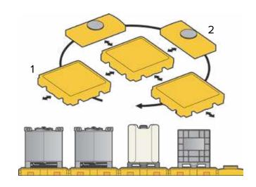
**Step 2:** Locate the two drill points on each mating sidewall of the (1) Pallet and/or (2) Expansion Tank. Note: the drill points are dimples in the sidewall that are located approximately 2 ½" from the bottom of the (1) Pallet or (2) Expansion Tank and are 18" apart.
